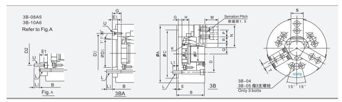
注:着色部分爲3BA型之寸法 The dimensions and the specifications of 3BA type are in the tinted area.
